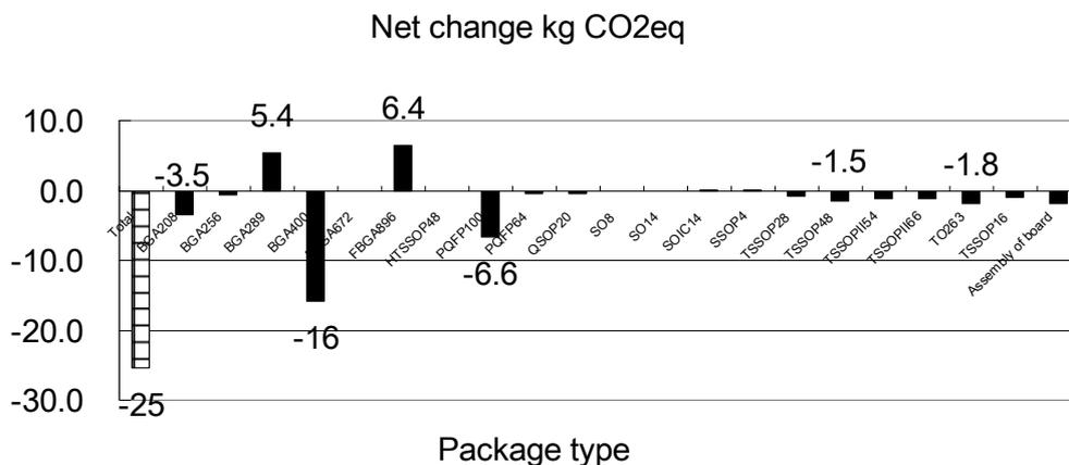
Note that the CO<sub>2</sub>e in Figure 3 is limited to ICs, with no other electronic components.
