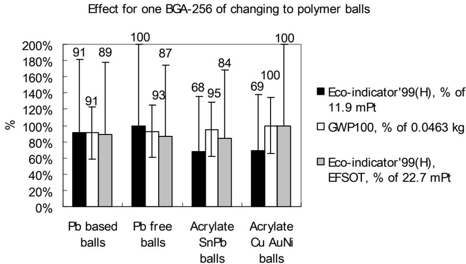
The acrylate Cu AuNi balls gave as result more detrimental environmental impact, as expressed with the indicator GWP100, compared with the acrylate Cu SnPb balls, in 95% of Monte Carlo runs.
