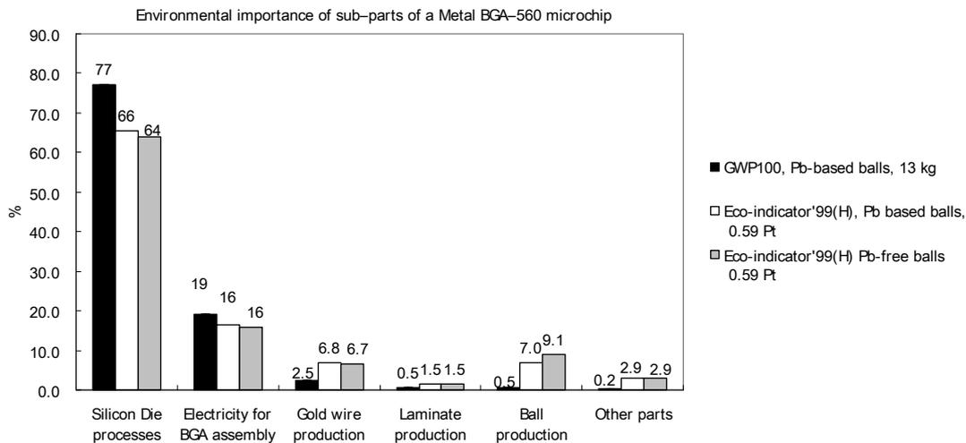
From the results of GWP100 and Eco–indicator’99 (H) shares of BGA–560 constituents a preliminary conclusion can be drawn that solder balls have small environmental impact for metal BGA–560 microchip packages. The shift to Pb–free ball material does not necessarily lead to environmental improvement.
