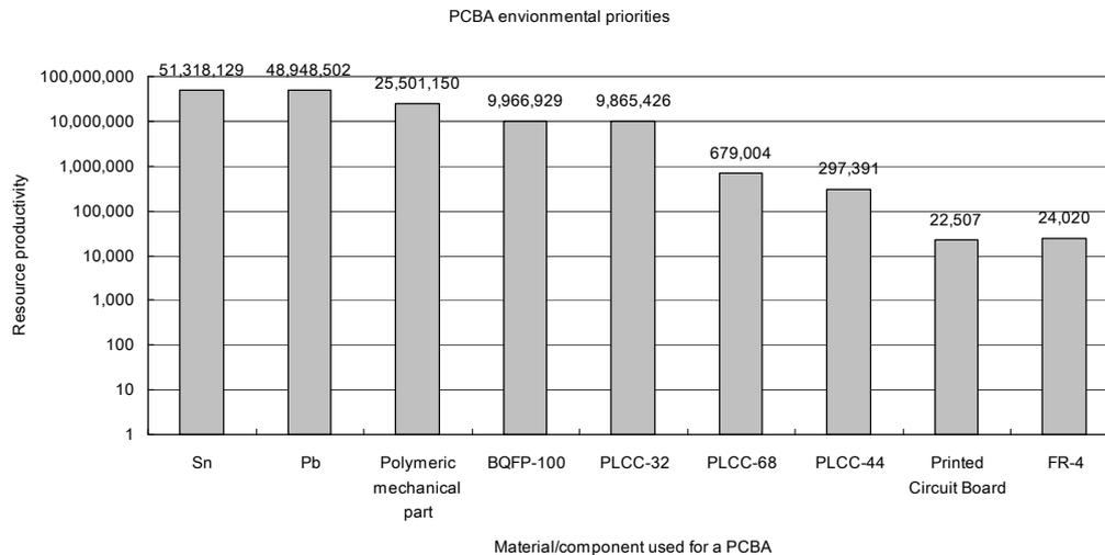
Alcatel–Lucent’s RP approach does not necessarily give different conclusions for PCBAs designers than plain process sum LCA. Most PCBA LCAs also show that the PCB and the ICs have a similar relation as in *Figure 13*.
