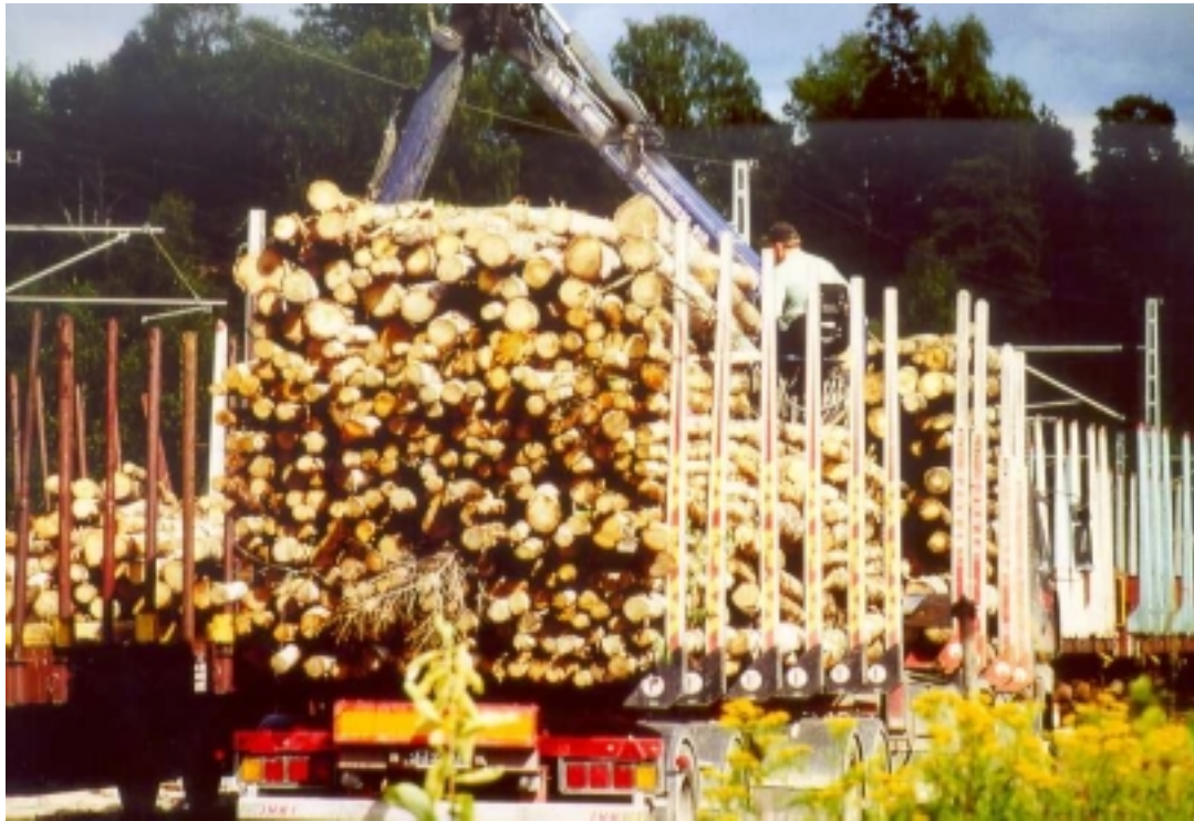
Figure 17 The reloading of logs from the lorry to the railway wagon (Foto:UPM-Kymmene 2000).
