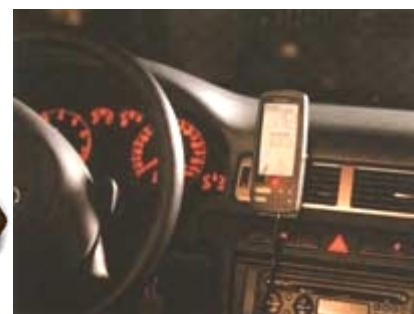
Figure 47 On-board device for fuel consumption measurement and training (Source: EcoDriving, 1999)
