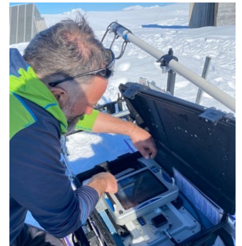
Ice radar measurements at Jostedalbreen Photo: K. Sjursen, JOSTICE-project, HVL.
