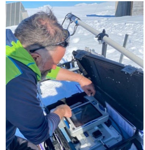
Ice radar measurements at Jostedalsbreen Photo: K. Sjørnsen, JOSTICE-project, HVL.
